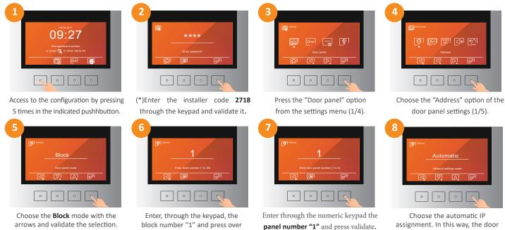
idate. assignment. In this way, the door panel will take the **192.168.100.101** IP address.
