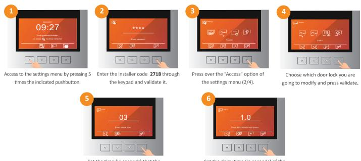
Set the time (in seconds) that the door lock will remain enabled.
