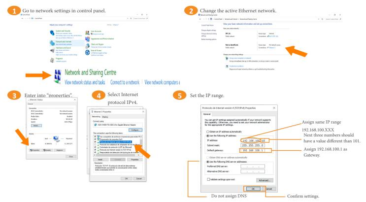
In this moment, the computer is ready to work in the same IP range as the panel IP address.
