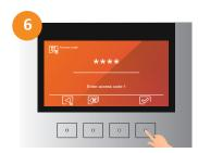
Enter the desired 4 digits access code and press validate. You must enter the first code and then the second one after validating the first.
