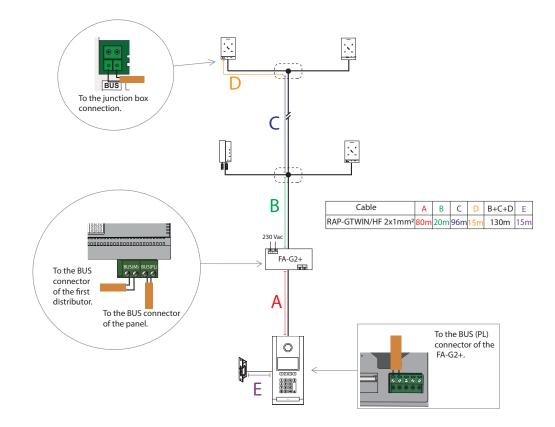
IN-OUT installation with 8 columns without distributors, maximum 16 audio units per column and 128 audio units in the installation. All the indoor units must have the DIP 10 in the OFF position. Make junction box connections.
