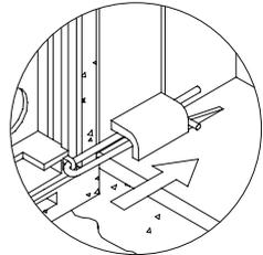
Link the sound module with the keypad module by using the supplied flat cable.
