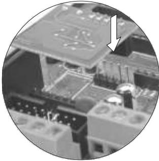
Optional. EL560 module for video installations with twisted pair cable.
