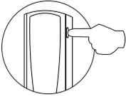
Press the door release push button and with this button pressed, pick up the handset.
