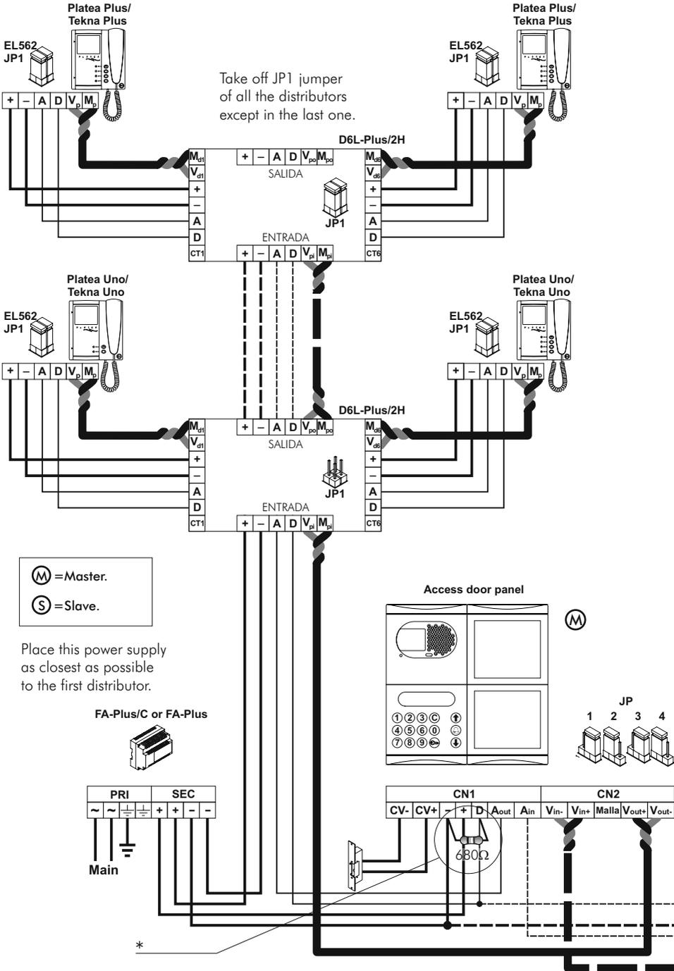
**V**ideo installation without coaxial cable and Plus/Uno monitors.
