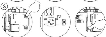
To programm the telephone as **Slave**, press the P1 door release push button (the telephone led will quick blink) and later press the hook switch (the led will off).
