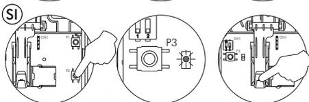
To programm the telephone as **Slave + Intercom.**, press the P2 auxiliary function push button (the led will quick blink) and later press the hook switch (the led will off).
