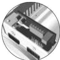
***In Platea/Tekna Plus:*** Locate the CN4 connector, that's placed in the monitor base. Remove the existing jumper and plug the EL562 module.
