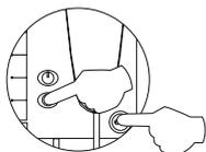
Keep the autoswitch-on button pressed and without releasing it, press the door opener button.
