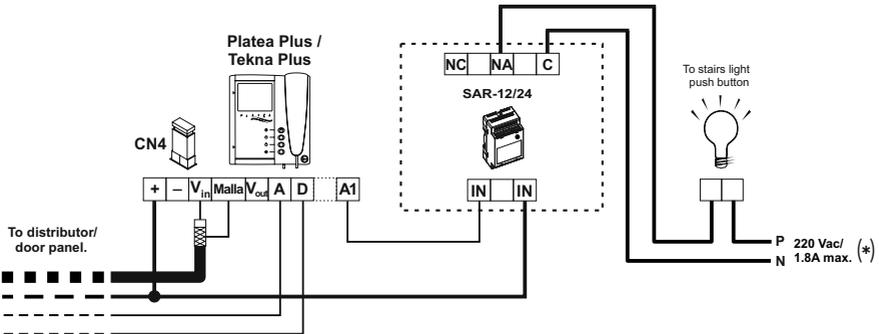
(\*) The neutral supply from the stairs light will be wired through the relay contacts SAR-12/24, the maximum current for stairs light will be 1.8A.
