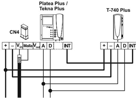
**\* IMPORTANT:** The T-740 Plus telephone must be configured with SW1 dip switch in "Intercom" mode function (see page 139).
