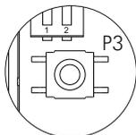
The P3 programm push button is located in the top part left of the circuit, it is accessed by opening the telephone. Allows to telephone enter in programming mode with the door panel, (see programming process on page 143).
