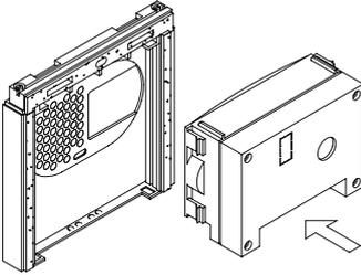
Insert the sound module in the grille module. For a proper assembly, align the light push button and the microphone rubber of the sound module with its corresponding holes in the grille module.
