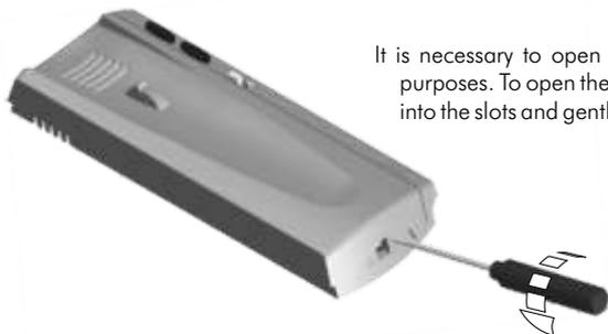
It is necessary to open the telephone for wiring and fixing purposes. To open the telephone, insert a plain screwdriver into the slots and gently lever as shown in the drawing.
