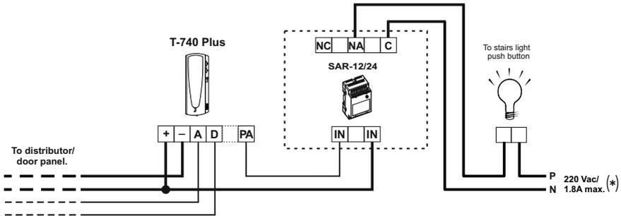
(\*) The neutral supply from the stairs light will be wired through the relay contacts SAR-12/24, the maximum current for stairs light will be 1.8A.
