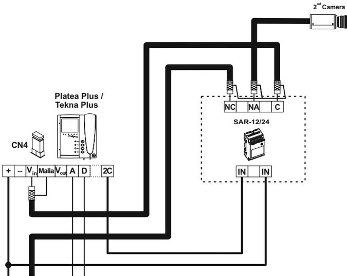
**E**xternal lock release activation with T-740Plus telephone.
