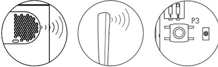
To show that the system is ready for programming, the panel and telephone handset will reproduce a sound (the telephone led will light and the LCD will display the message *pr o g r a m* mode). Audio communication can be established.
