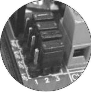
The JP1, JP2, JP3 and JP4 configuration jumpers are placed on the left side of the terminal connector.
