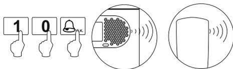
Enter the code of the monitor to be programmed and press the
