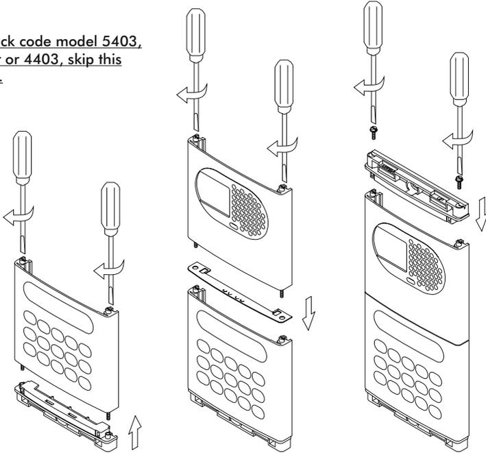
Insert the header DOWN marked in the lower module and fix it by screwing the module shafts.
