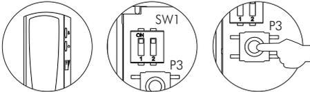
Open the telephone to programming (see page 140). Select in the SW1 dip switch the function mode for the auxiliary function push button (see page 139) and later press the P3 programming push-button.
