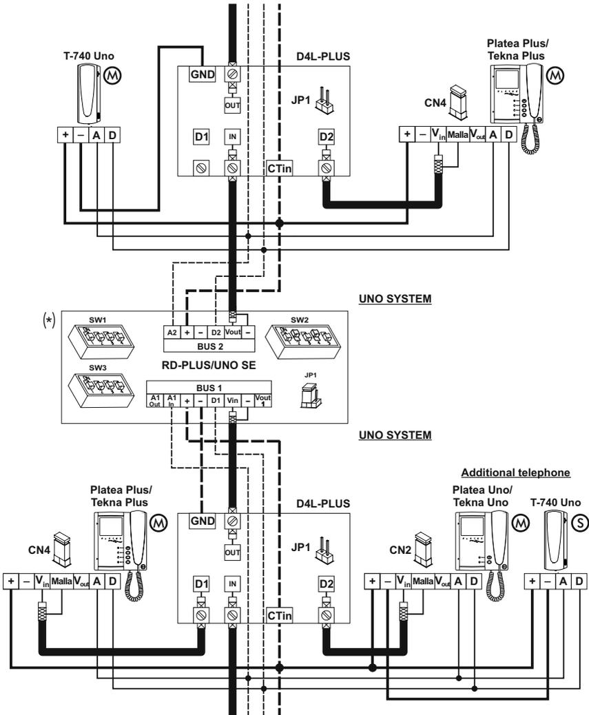
(\*) Important: For the connection and configuration of the RD-PLUS/UNO SE, see the TRD-PLUS/UNO SE manual).
