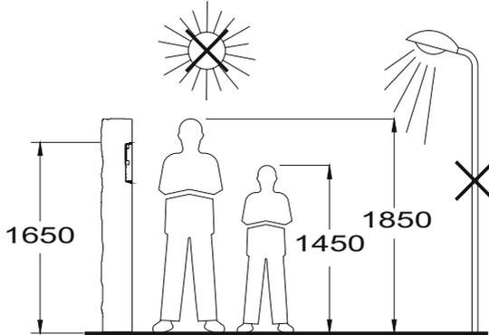
The upper part of the door panel should be placed at 1,65m. height roughly. The hole dimensions will depend on the number of door panel modules.
