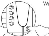
With the door release push button pressed switch on the monitor.
