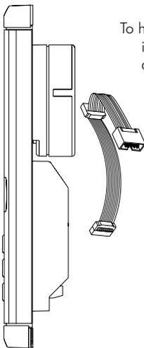
To hold the door panel on the embedding box, insert the hinges in the embedding box lockers as shown.
