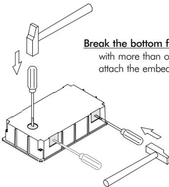
**Break the bottom flange** to pass the cables through. In case of door panels with more than one embedding box, break the side flanges and attach the embedding boxes using UC junctions.
