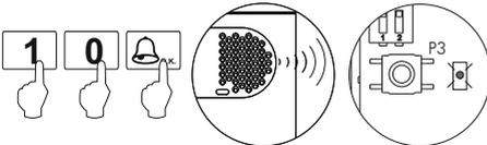
Enter the code that will be used to call to this telephone and press the key. At this moment the panel and telephone handset will reproduce a sound (the telephone led will slow blink).
