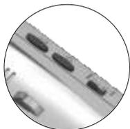
☞ If the handset is on the cradle sends a panic call to the porter's exchanges that have enabled the reception of this type of call. If not, allows to call to the master porter's exchange. During call reception and communication progresses allows the lock release activation.
