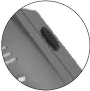
If the handset is off the hook, allows to call to the master porter's exchange.
