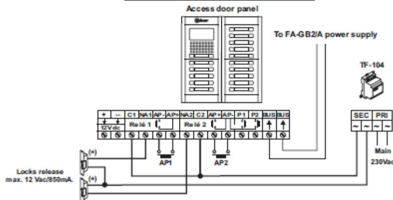
(+)Important: Place the varistors supplied with the sound module on each lock release terminals directly to ensure a proper system operation.
