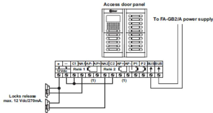
(!)Important: Do not use the "AP" push buttons door release if there are connected 2 d.c locks release.
