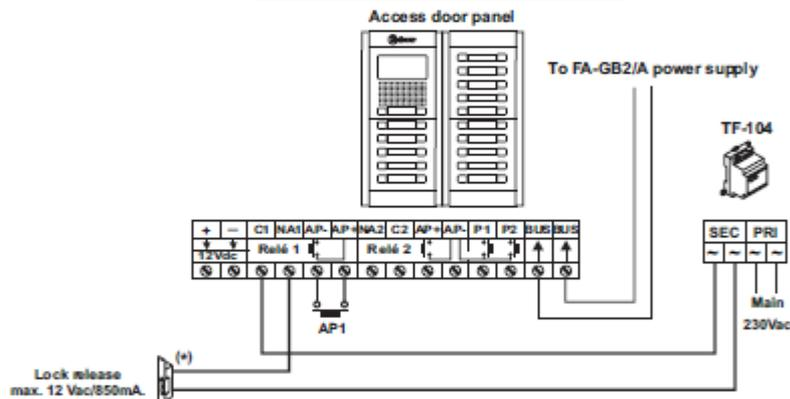
(+)Important: Place the varistor supplied with the sound module on the lock release terminals directly to ensure a proper system operation.
