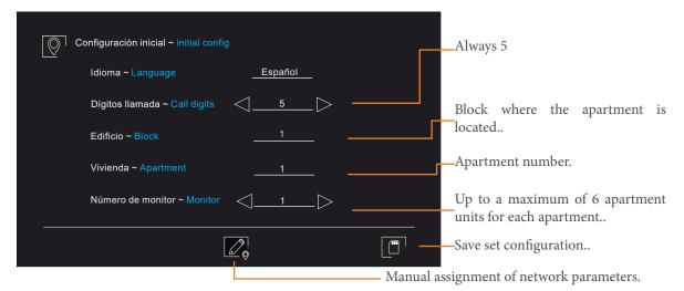
If you want to assign different network parameters to which the ones that automatically assigns the system, we must press the located on the bottom of the screen. This will bring us to another screen that will request to enter the desired network parameters.
