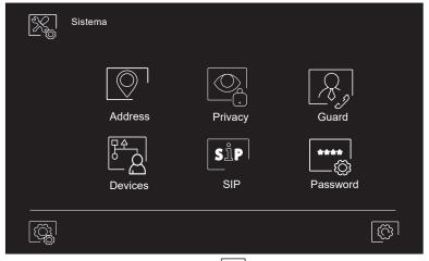
To return the monitor settings to factory values, we must press on the [ icon located on the bottom right in the screen. It will appear the following screen and we must confirm the restore to factory values of the monitor settings.
