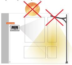
2- Place the top of the monitor at a height of 1,65m for a correct viewing of the screen:
