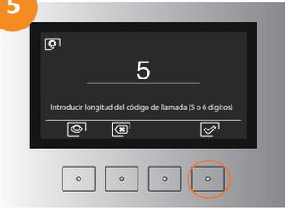
5 Select 5 digits dialling length. \*6 digits dialling code length in the case you like to indicate the floor
