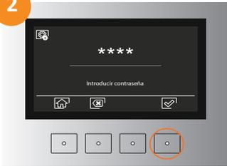
2 Type the installer PIN code "2718" with the keypad and press validation
