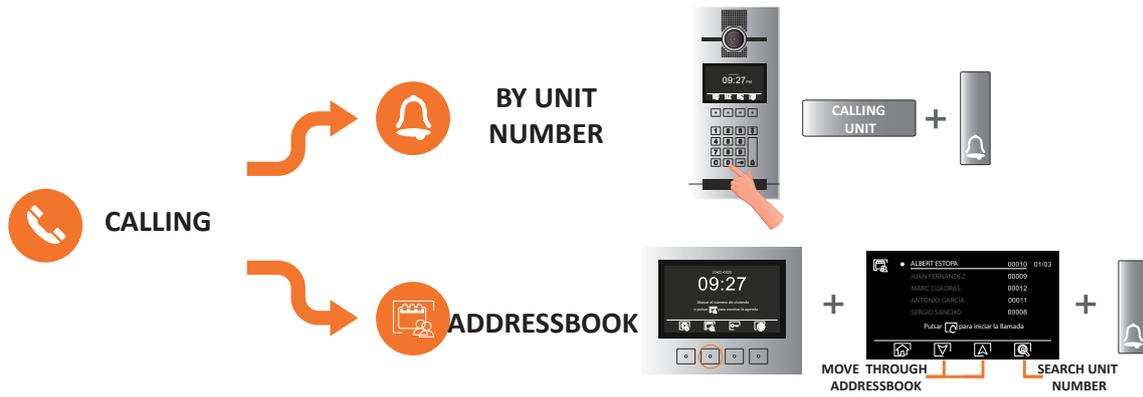
The call process lasts for a maximum of 45 seconds. The panel will prompt the voice message "call is in progress" and will display that message on screen. If after 45 seconds the call has not been answered, it will indicate "No response, try it later".
