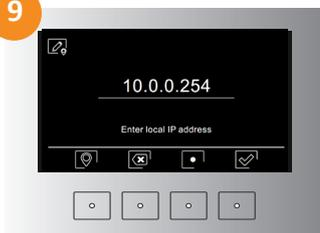
9 Enter the desired IP address of the panel and press validation icon.
