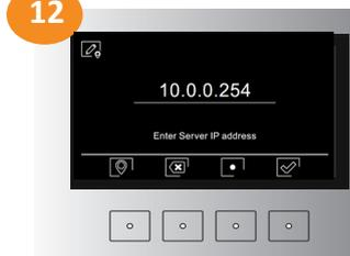
12 Enter the IP Server address. It is **IP address** of the **system manager panel**.
