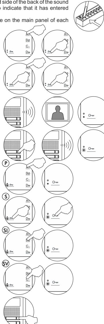
Press and hold door release button  $G\leftrightarrow$  and, without releasing it, switch on the monitor (press button  $A\downarrow$  for 1 second).
