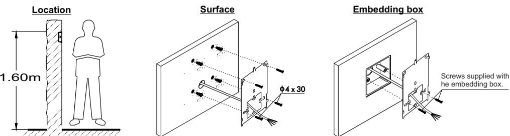
Remember to remove the protective covering from the front of the monitor once installation is complete.
