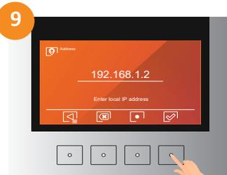
9 Enter the desired IP address for the door panel and press validate.
