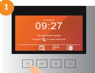
1 Access to the configuration by pressing 5 times in the indicated pushbutton.
