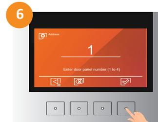
6 Enter through the numerical keypad the number of **general panel** and press validate
