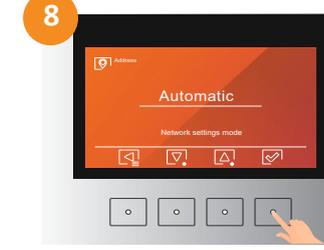
8 Choose the automatic IP assignment. In this way, the door panel will take the **192.168.100.101** IP address.
