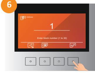
6 Enter, through the keypad, the block number "1" and press over the validate option.
