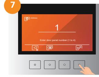
7 Enter through the numeric keypad the **panel number "1"** and press validate.
