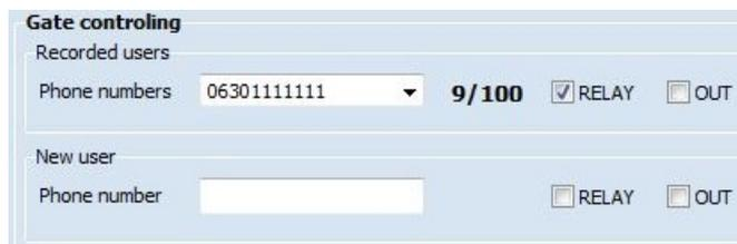
When calling the intercom from the phone numbers specified here, control of the output or outputs assigned to the given phone number is performed. The incoming call is not accepted from the configured telephone number, so this function operates with a free call. Maximum 100 user phone numbers can be added.
