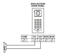
If the lock release to be used is alternating current, use a relay and transformer suitable for the consumption, as well as the varistor supplied. The example shows a Golmar SAR-12/24 relay and a TF-104 transformer (12Vac/1.5A).
