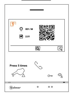
The 'special codes' screen will then be displayed. Press the button below icon  $\bigcirc$  to select the field to be modified and press the buttons below icons  $\bigcirc$ / $\bigcirc$ /to enter the desired code. Once the code has been entered, press the button below icon  $\bigcirc$ / to validate it. If the code entered is valid, icon  $\checkmark$  will be displayed; if it is not, icon X will be shown.
