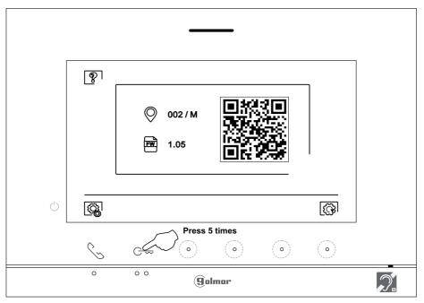
The 'special codes' screen will then be displayed. Press the button/ hidden button below icons  $\boxed{}$  /  $\boxed{}$  to select the field to be modified and press the hidden buttons below icons  $\boxed{}$  /  $\boxed{}$  to enter the desired code. Once the code has been entered, press the hidden button below icon  $\boxed{}$  to validate it. If the code entered is valid, icon  $\checkmark$  will be displayed; if it is not, icon  $\boxed{}$  will be shown.
