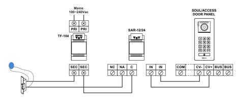
**Important:** More than 2 access door panels, DPM-G2+ multiplexer required and AC lock release must be connected to door panels 3 and 4 (instead of DC lock release) with a SAR-12/24 relay module and a TF-104 transformer.
